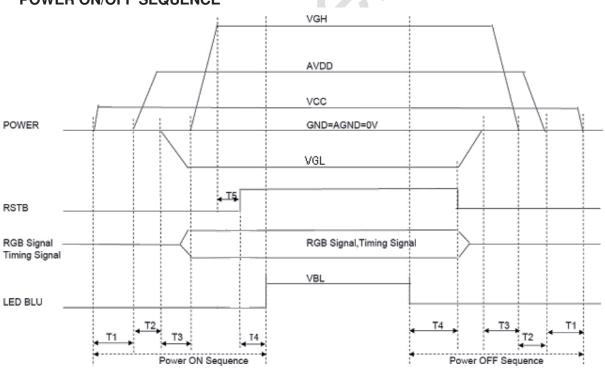
Note 1: T1≥20ms, T2≥20ms, T3≥5ms, T4≥100ms, T5≥5ms.
