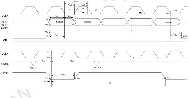
Figure 6.1.1 Clock and Data Input Timing Diagram
