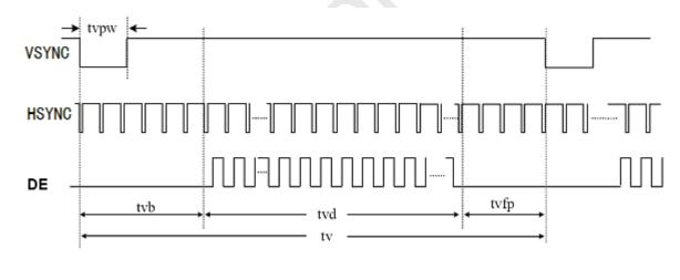
Figure 6.3.1 TCON Vertical Input Timing Diagram HV
