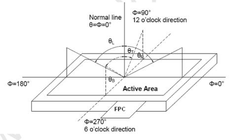
Fig2. Measurement viewing angle
