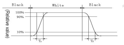
Fig4.Response Time Testing(SFT)
