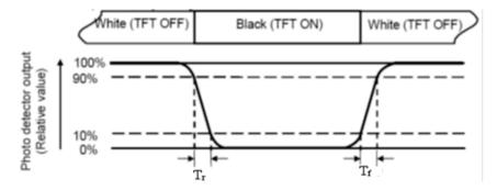
Fig3. Response Time Testing(TN)
