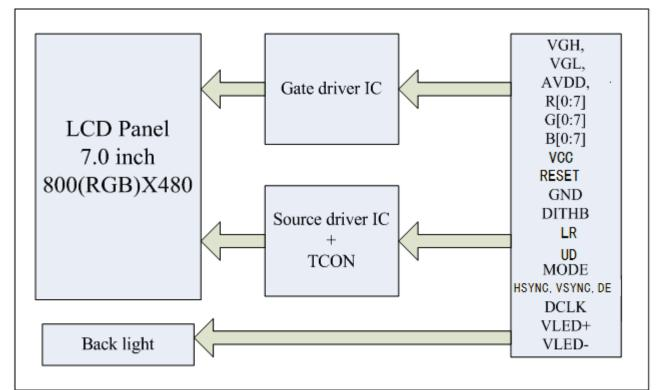
Figure 5.5.1 LCD Module Block Diagram
