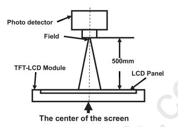
Fig1.Measurement Set Up
