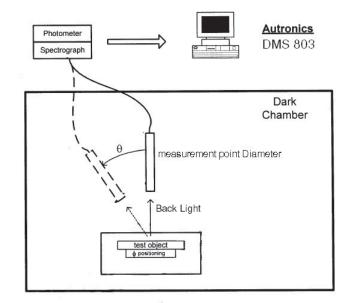
Fig. 4-2 Optical measurement system setup
