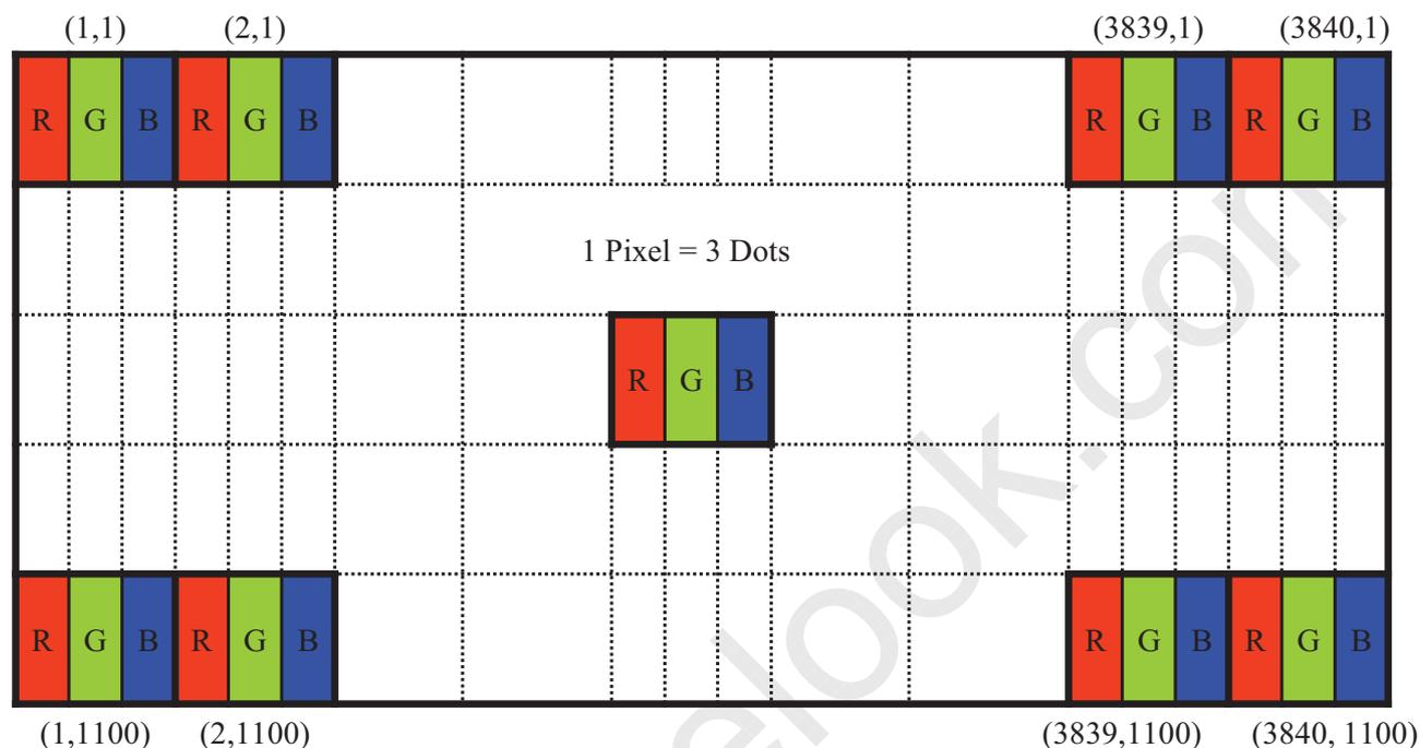
Figure 13. Display Position of Input Data (V-H)
