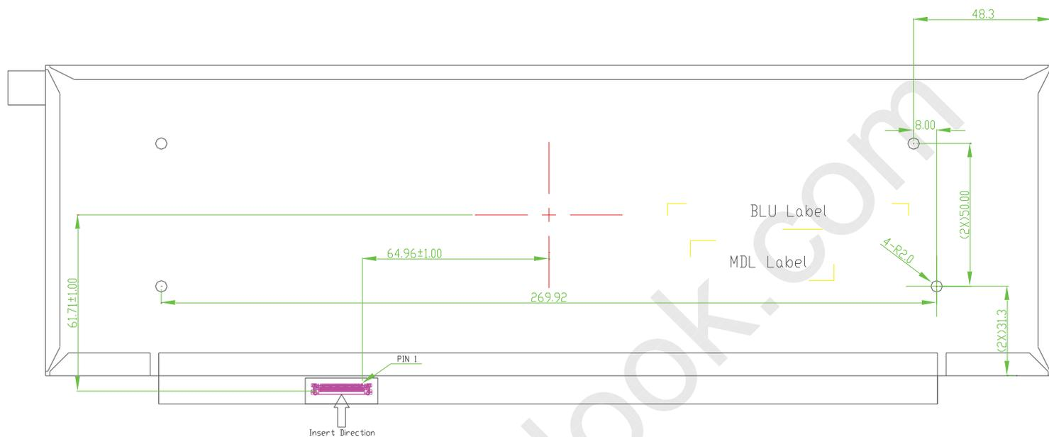
Figure 26. TFT-LCD Module Outline Dimensions (Rear view)
